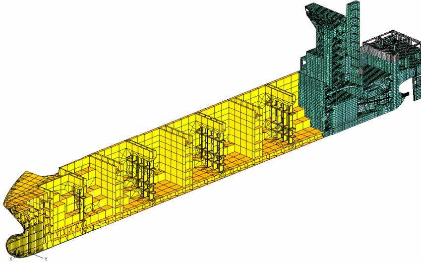
Figure 1: The structural finite element model of the container ship.
