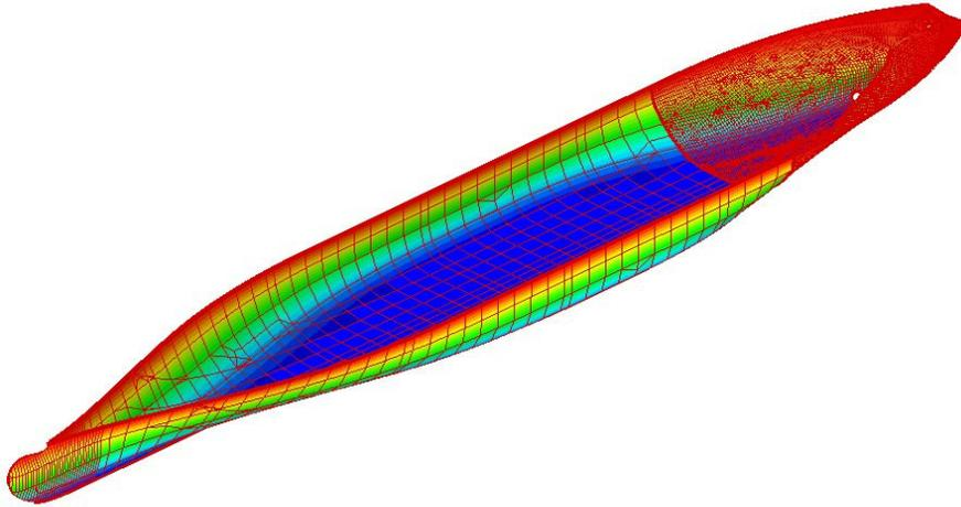
Figure 2: The discretized wetted surface of the container ship for the full load condition.
