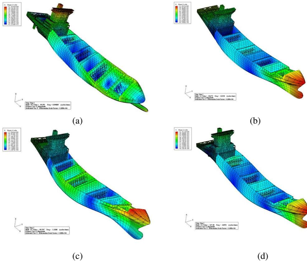
Figure 3: The first four global modes of the container ship: (a) 1<sup>st</sup> torsion, (b) 1<sup>st</sup> bending, (c) horizontal bending & torsion, (d) 2<sup>nd</sup> bending.
